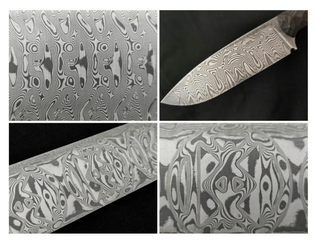
**#FFMARTENSITE** is a stainless damascus steel, where we combine two high-performance martensitic steels UHB AEB-L + UHB SS716. Our production of damascus steel is a highly controlled process, made under high pressure in a protective atmosphere.
