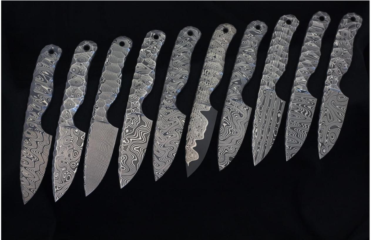
**#FFCONTRAST** is stainless damascus steel with a high-contrast. We combine high performance martensitic steel UHB AEB-L with austenitic AISI 304. Our production of damascus steel is a highly controlled process, made under high pressure in a protective atmosphere.
