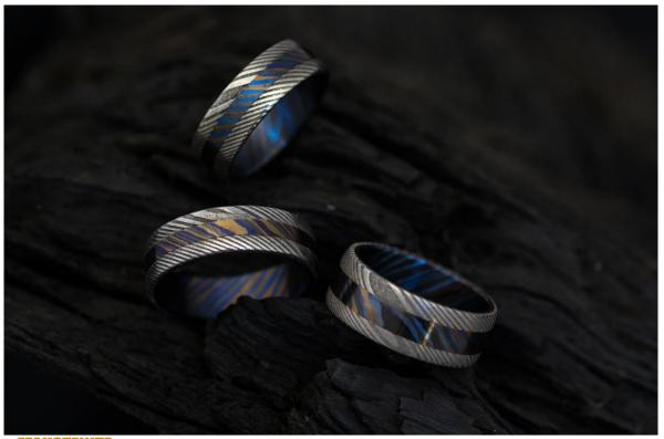
**#FFAUSTENITE** is a stainless damascus steel made of two austenitic (non-hardenable) steels AISI 304 + AISI 316. Our production of damascus steel is a highly controlled process, made under high pressure in a protective atmosphere.
